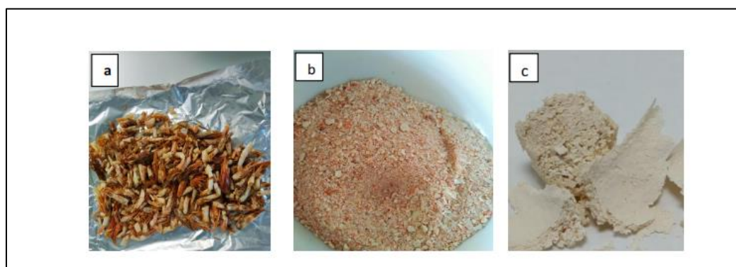
Figure 3 (a) Shrimp shells (b) after drying and grinding (c) chitosan
